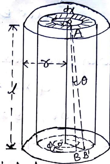
the angle of shear  $\theta$  for this shell. In the curved triangle  $OB\dot{B}'$ , we have
